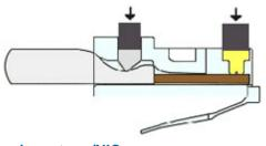
wedge onto the cable jacket and very firmly clinches it. The other seats the "pins," each with two teeth at its end, through the insulation and into the conductors of their respective wires.
