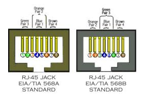
Note that pPins 4, 5, 7, and 8 and the blue and brown pairs are not used in either standard. These pins and wires are not used or required to implement 100BASE-TX duplexing—they are just plain wasted. Some people use want to 'save' these wasted wires and attempt to use them to carry voice or other data.
