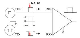
Pulses of energy travel down the transmission line near the speed of light (186,000 miles/ second). The principal components of one of these pulses of energy are the voltage potential between wires and current flowing near the surface of the wires.
